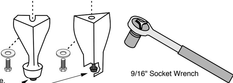
These rubber-tipped bolts are for leveling the stove. Make sure they contact the floor. Do not adjust with weight on the legs, the rubber tips may tear.
