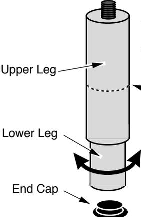
**A** Insert the end cap into the lower leg
