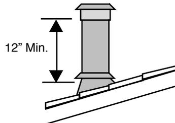
**Note:** ANSI 223.1, section 7.6.2 outlines additional requirements for gas vent terminations. If your installation involves a roof with a slope greater than 6/12 or if a wall or other vertical obstruction is within 8' of the vent termination, the vent termination will need to be taller. Refer to ANSI 223.1 for full details.
