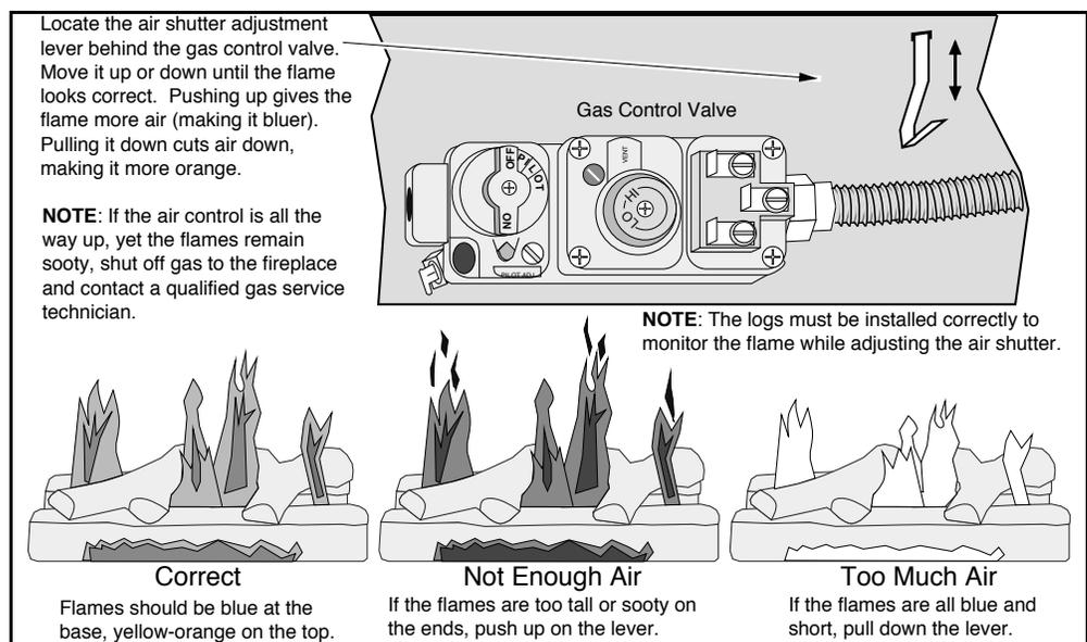
! If the air shutter is in its fully open position, yet the flames remain sooty, shut off gas to the heater and contact your dealer for a remedy.
