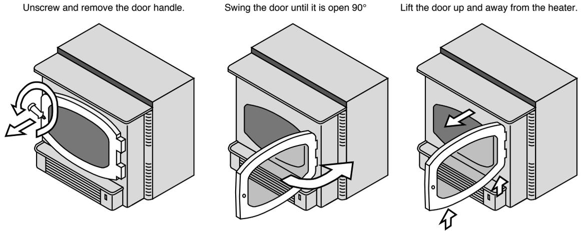
NOTE: When re-installing, make sure the handle points away from the glass when finished.
