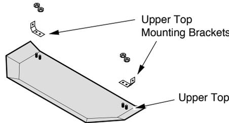
**WARNING:** Do not over-tighten the nuts, this may cause the enamel to chip or crack.
