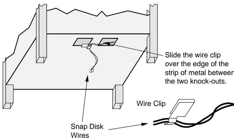
Feed the two snap disk wires into the eye of the wire clip. Remove all slack from the wire, making sure not to dislodge the snap disk. Pinch the eye of the wire clip to secure the wires.
