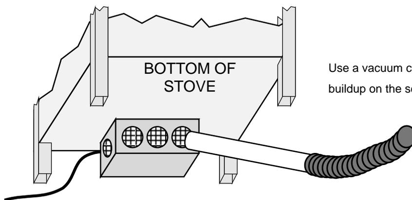
Use a vacuum cleaner to remove any buildup on the screens of the blower.
