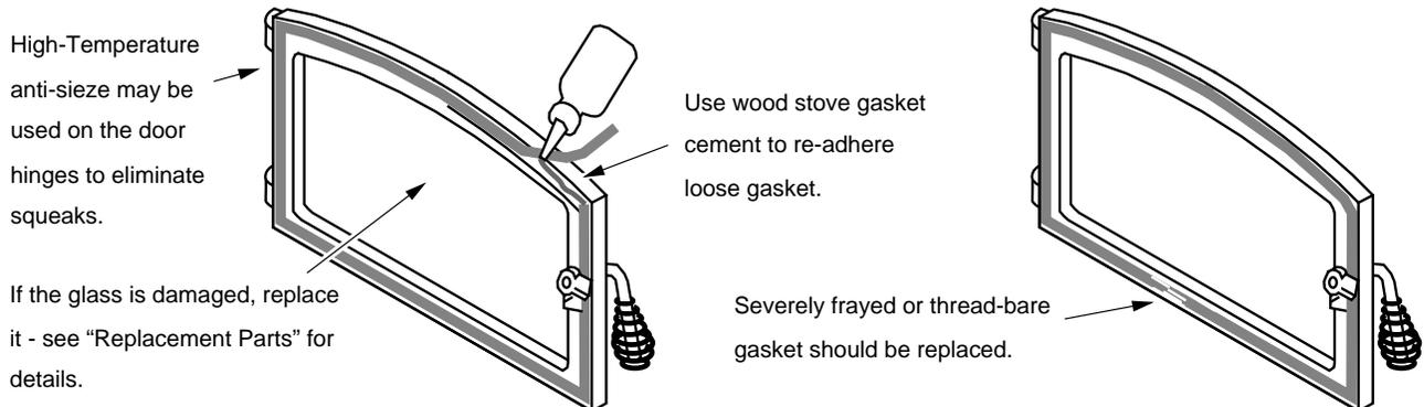
The door latch should pull the door against the face of the stove (but not so tight as to not allow full handle rotation). If the latch requires adjustment, follow the directions below.
